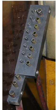
Manifolds in the piano (bass end)
