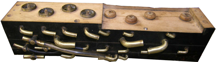
Above: The valve block. Left four valves are theme primaries, centre two are for tracking, right two for reroll, motor off.
