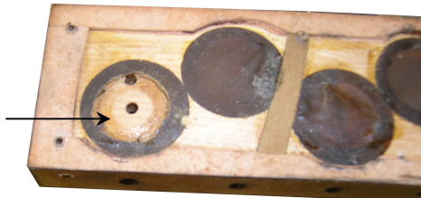
Above: The valve block. Left four valves are theme primaries, centre two are for tracking, right two for reroll, motor off.
